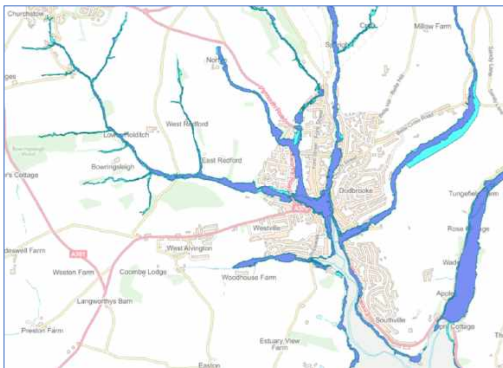
Figure 20A Environment Agency Fluvial Flood Risk Areas Zone 2 light blue, Zone 3 dark blue
