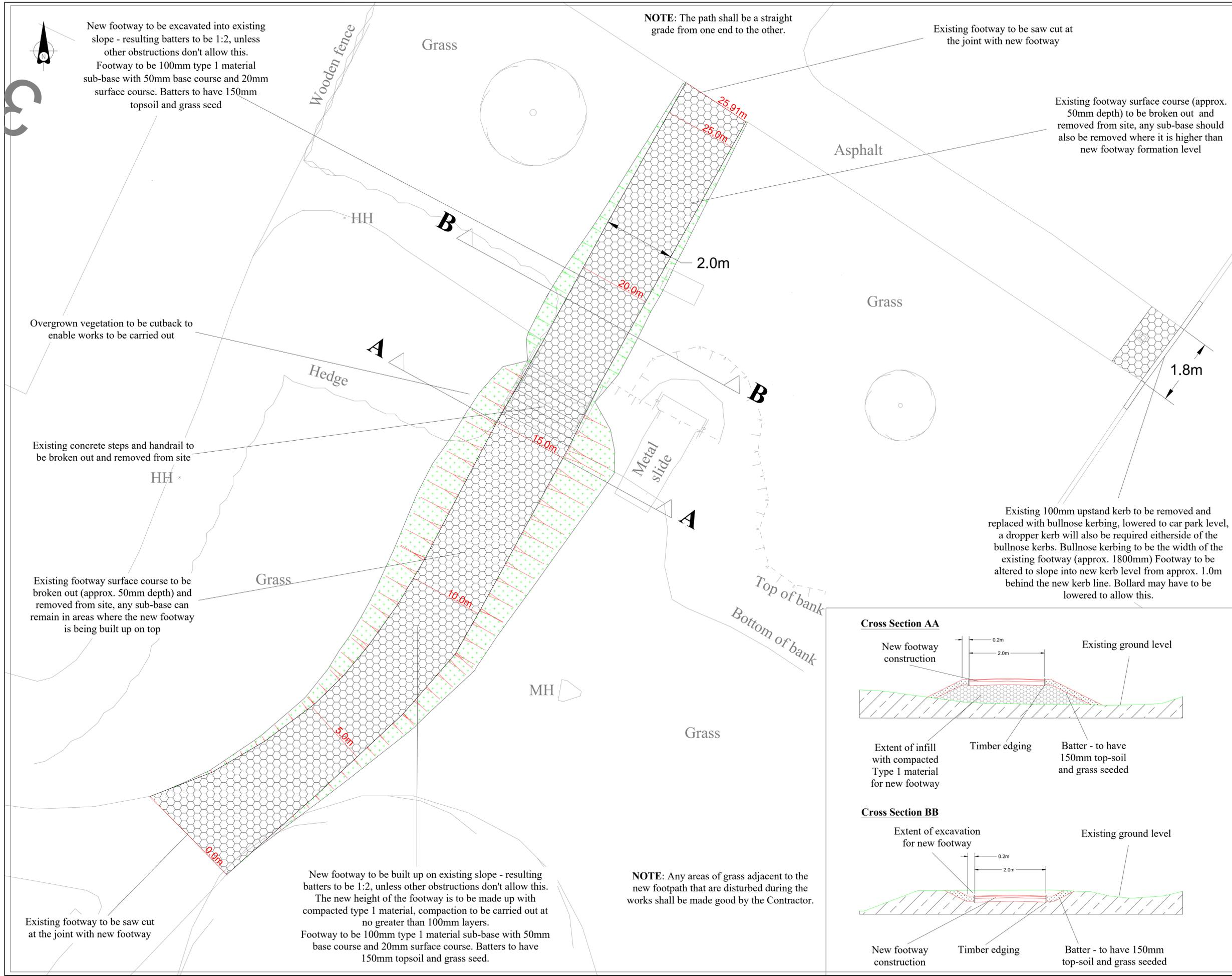
New footway to be excavated into existing slope - resulting batters to be 1:2, unless other obstructions don't allow this.
